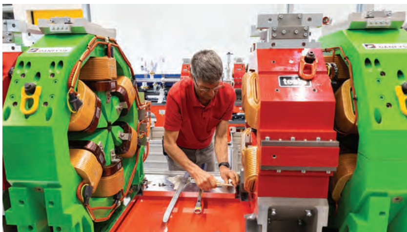
Fig. 2: Over 1000 new magnets have now been constructed, received and tested, including 132 permanent magnet dipoles and 983 innovative electromagnets, including sextupoles (left, green) and high-gradient quadrupoles (right, red).
