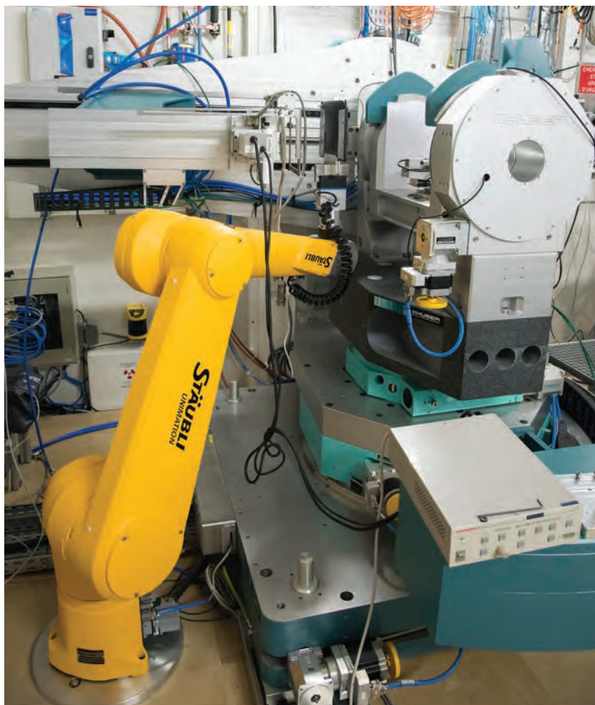
Fig. 146: The IRT diffractometer and robotic sample changer have sped up topography experiments at BM05, increasing its attractiveness for industrial clients.
