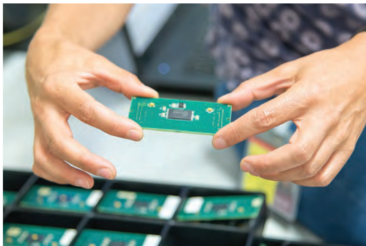
Fig. 147: The 3D stacked memory devices from satellites tested on ID09 for resistance to radiation.
